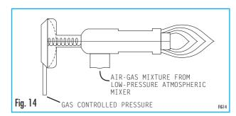
move forward. In this way the free section of the central port of the nozzle will be be increased. The disc is free to run for up to 40 mm. From its maximum forward position, the disc will run the whole way back entrained by the spring tension as the gas boost decreases. Burners equipped with this device may reach capacity ratios higher than 10/1 even with maximum gas pressures of 150 mm  $H_20$  and in medium draft conditions. With higher gas pressures higher capacity ratios may be obtained.
