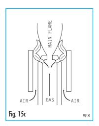
nozzle; otherwise the pilot flamelets will blowoff and the effect of flame holding would disappear.
