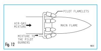
In some sophisticated, expensive industrial processes, the mixture is supplied to the flamelets, called "pilot" flamelets, by a mixer and a conduit which are completely separated from those of the main burner (fig. 12).
