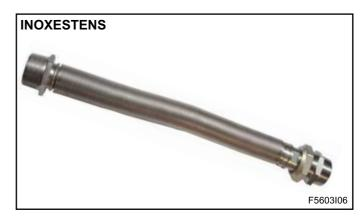
When these hoses are used to connect non-aligned tubes, the mounter will have to bend them slightly before installation so that no force is applied to the burner or to the piping during tightening of the flange or fitting. The **INOXESTENS** series represent a type of extensible threaded joints in non-woven stainless steel. These flexible models are delivered with end fittings chosen according to the required junction (fixed or revolving).
